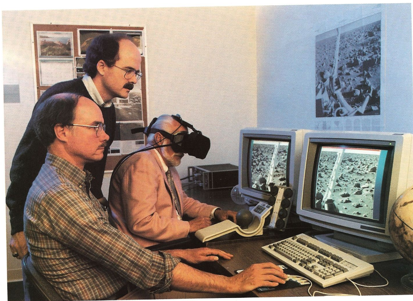
Figure 8. Creation of a virtual environment offers another alternative to personal presence in space. With digital imagery and other data gathered by robotic missions, it might be possible to construct a virtual planetary surface—one that exists only as a computer model—that an earthbound astronaut could wander over at will. The user typically wears a head-mounted stereoscopic display, which the computer operates in such a way that the scene changes appropriately as the user moves his or her head. The device shown here is the Virtual Planetary Exploration system developed at the NASA Ames Research Center by Michael W. McGreevy ( standing ) and his colleagues, one of whom is wearing a head-mounted display. The two monitors show the two slightly different images of the Martian landscape that are being projected within the goggles. The imagery comes from the Viking 2 lander. McGreevy and his colleagues have observed and interviewed planetary geologists to determine how they do field work and are currently attempting to design interface modes that will accommodate the geologists' needs.
