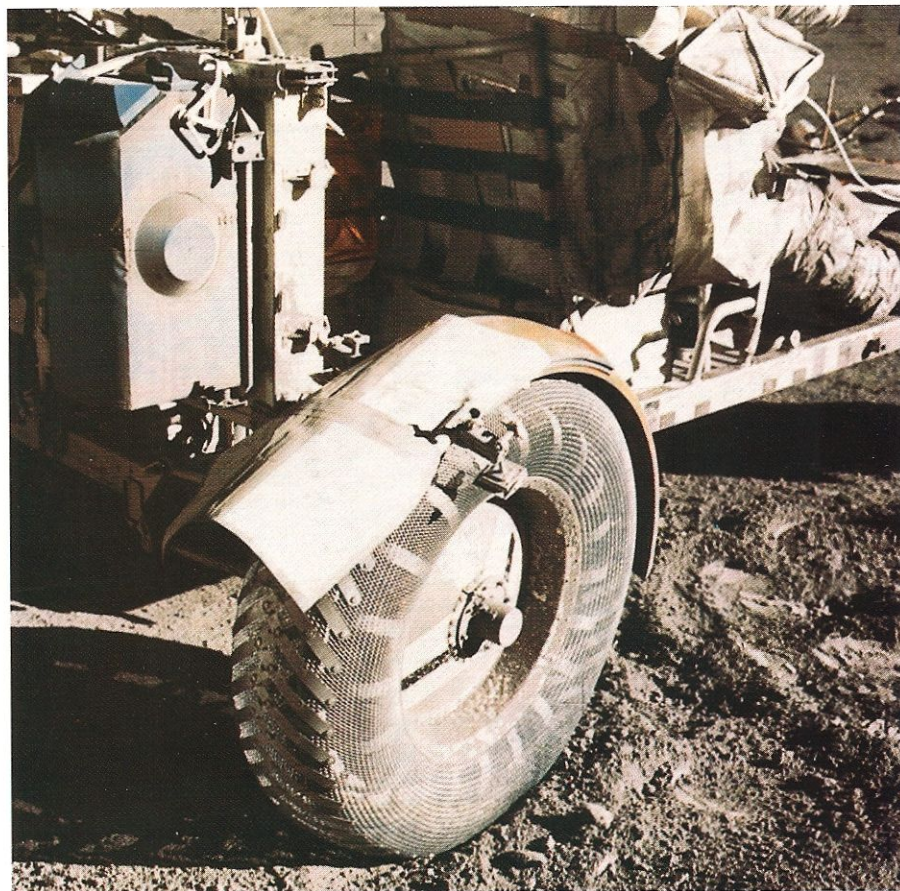
Figure 5. Fragile fender of the Apollo Lunar Rover provides an example of the ingenuity people bring to repair work. The commanders of the last three Apollo missions each broke a fender on the Rover. With the fender missing, the wheel sprayed lunar dust over the vehicle, which was more than a nuisance: By coating optical and electronic equipment, it could have curtailed exploration. A replacement fender was fashioned out of spare maps held by clamps.
